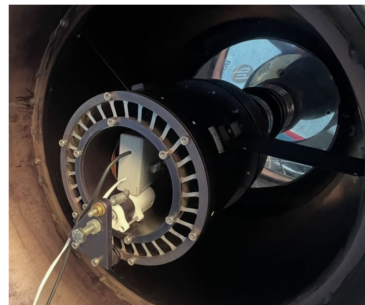
Figure 3: Interim focusing mechanism for ROTSE-IIIc, replacing the original micrometer with a linear actuator housed in a custom 3D-printed mount.
